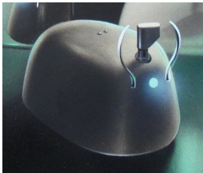
Figure 1. ELSIE: Electro-mechanical robot, Light Sensitive with Internal and External stability. Her scanning turret contains a single photo-cell, and a tilt of her shell detects contact with obstacles.
